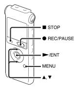
You can set the VOR (Voice Operated Recording) function to "ON" when the IC recorder is stopped or is recording, to make the IC recorder start recording when the IC recorder detects sound, and pause when no sound is heard, eliminating recording during soundless periods.
